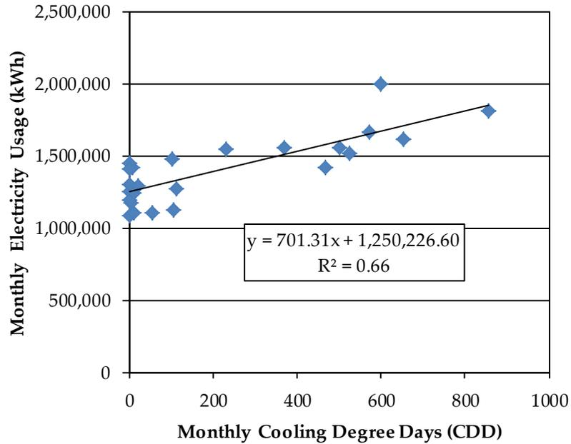
Figure 17: Monthly Electrical Usage vs. Cooling Degree Days (CDD)
