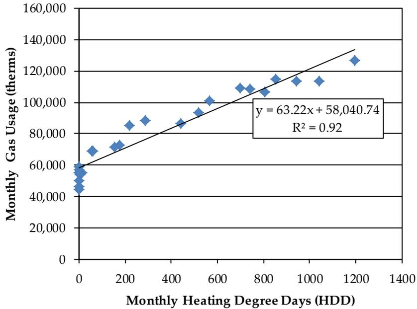
Figure 24: Monthly Natural Gas Usage vs. Heating Degree Days (HDD)
