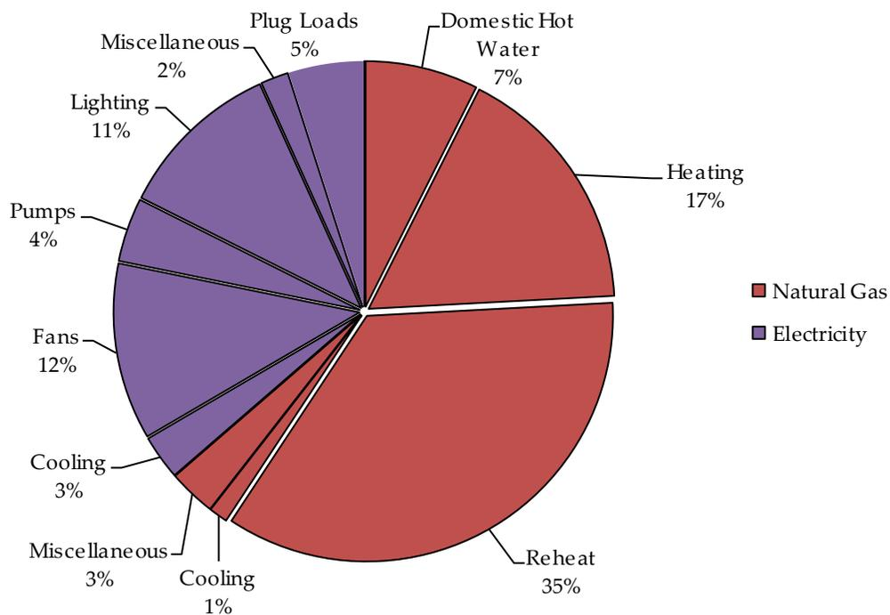
**Figure 14: Energy End Usage Breakdown**
